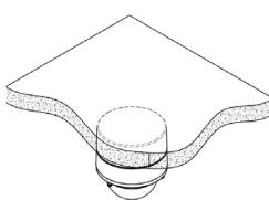
1. Use the mounting template to drill the mounting holes in the desired position.
