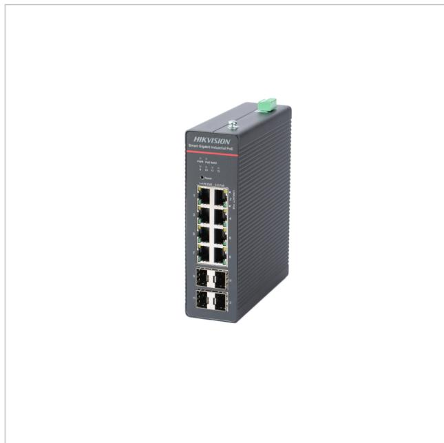
Ethernet Switch, Smart Managed, 8x Gigabit PoE RJ45, 4x Gigabit SFP Ports, 802.3bt Hi-PoE, 75W PoE
