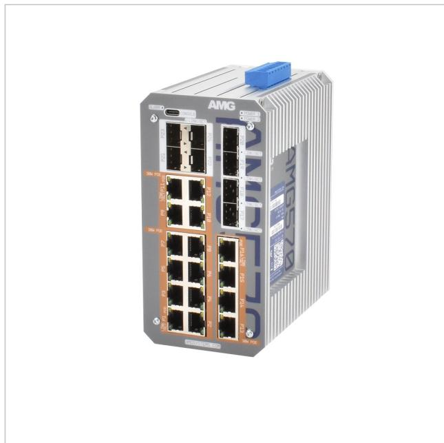
Industrieller 24 Port Managed Switch, 16 x 10/100/1000BT RJ45 mit 30W PoE, 2 x 100/1000/2,5GFX SFP Slots, 6 x 100/1000Base-FX SFP Slot
