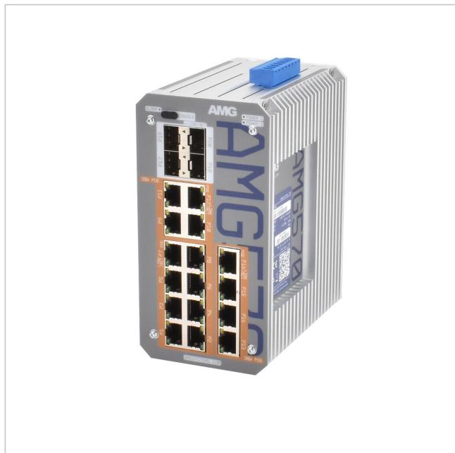
Industrieller 20 Port Managed Switch, 16 x 10/100/1000BT RJ45 mit 30W PoE, 2 x 100/1000/2,5GFX SFP Slots, 2 x 100/1000Base-FX SFP Slot
