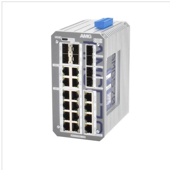
Industrieller 24 Port Managed Switch 16 x 10/100/1000BT, 2 x 100/1000/2,5GFX SFP Slot, 6 x 100/1000Base-FX SFP Slot, -40°C to +75°C
