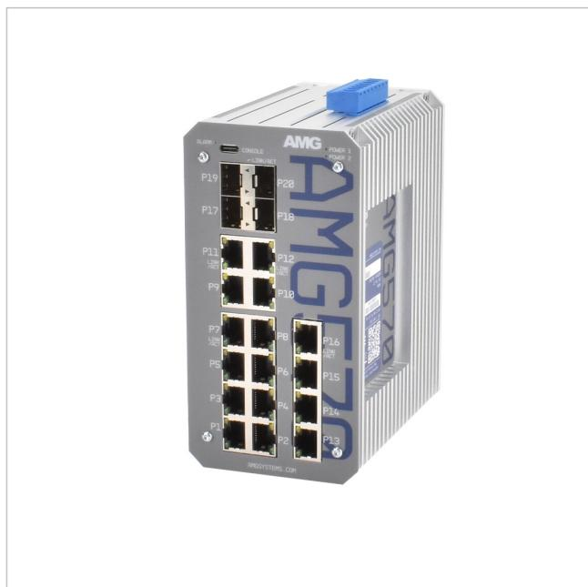
Industrieller 20 Port Managed Switch 16 x 10/100/1000BT, 2 x 100/1000/2,5GFX SFP Slot, 2 x 100/1000Base-FX SFP Slot, -40°C to +75°C
