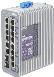
Industrieller 16 Port Unmanaged Switch, 14 x 10/100/1000BT RJ45 30W & 2 x 100/1000FX SFP Slot
