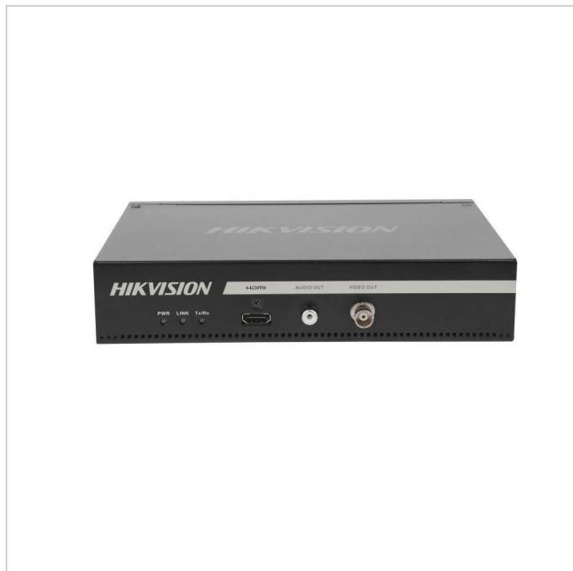
Video Decoder, 1-Kanal, 12MP, H.265, HDMI, VGA, FBAS
