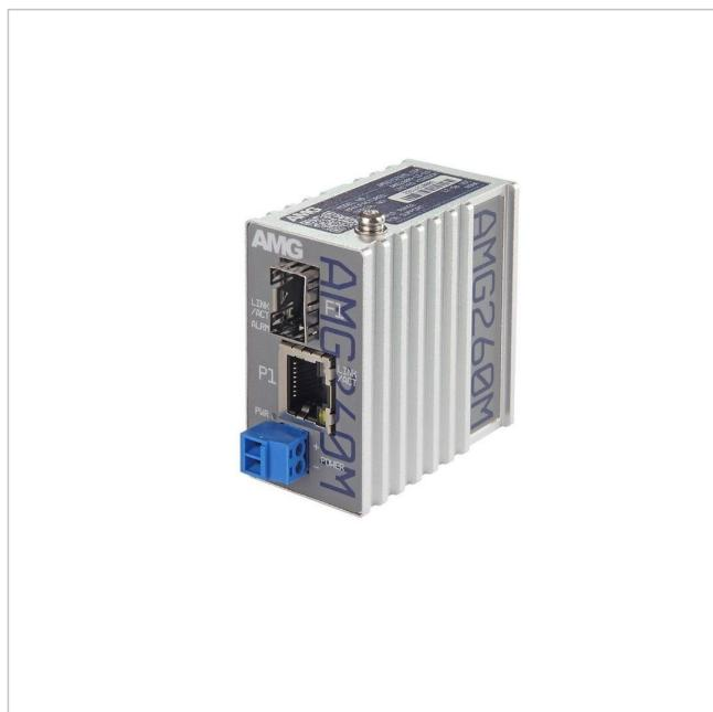
Industrieller Mini Medienkonverter, 1 x 10/100BT RJ45 , 1 x 100/1000FX SFP Slot, ohne SFP, DIP Switch, DIN Rail / Wandmontage
