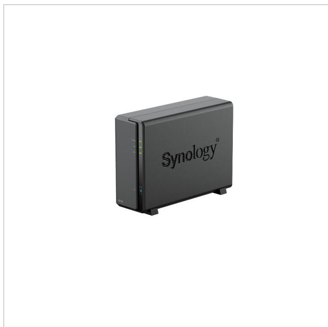
Network Attached Storage, 1-Bay, ohne HDD, 1x GBit LAN, 2x USB 3.0
