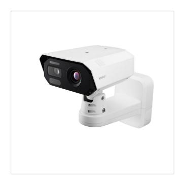
Bi-Spektrum KI-Wärmebildkamera, VGA 13,5mm, 8M Motorized 10,9-29mm, IP66/IP67, IK10, NEMA4X
