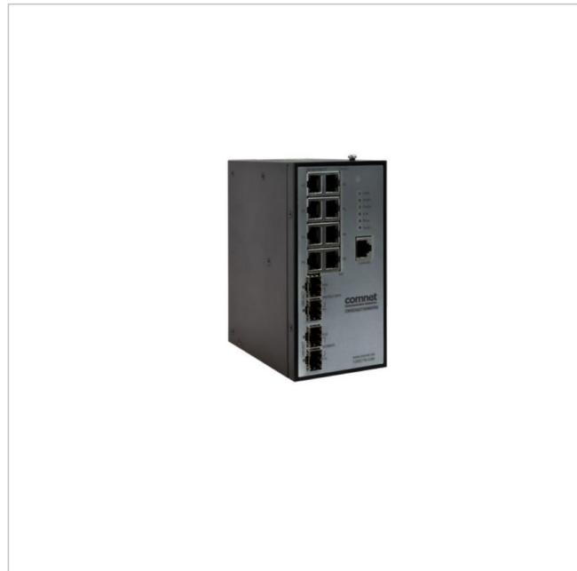
Ethernet Switch, managed, 8x RJ45 Gbit, 10G SFP
