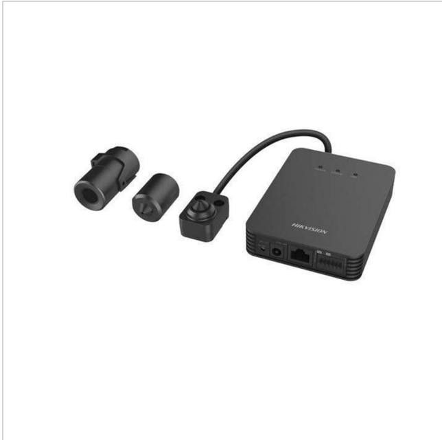
1/2.7" Netzwerk Kamera, Covert 1920x1080, PoE, WDR, 1,39mm, Turret Bracket, 8m Kabel
