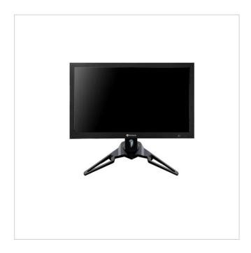
28" (72cm) LCD Monitor, 4K UHD, 3840x2160, 60fps, LED, Display Port, HDMI, DVI-D
