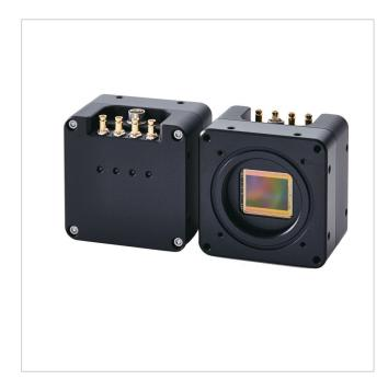
1,76" CoaXPress Kamera, Farbe, 12 Megapixel, 180fps, M42-Mount, Anschluss hinten
