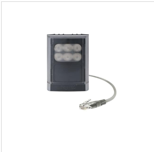
LED Infrarot Scheinwerfer, 940nm, 10x10, 35x10, 60x25, 12W, IP66, PoE
