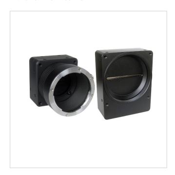
Dual Line, S/W Zeilenkamera, 4k, CMOS, 7µm, 160kHz, Camera Link, M42-Mount
