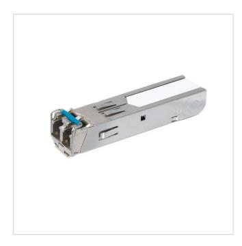
SFP Mini-GBIC Transceiver, Multi Mode, 2 Fiber, 1000Base-SX2, 2km
